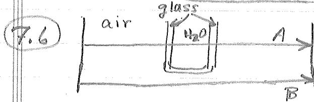
Optical path length of A  $\equiv$   $OPL_A = \sum_i n_i d_i$
